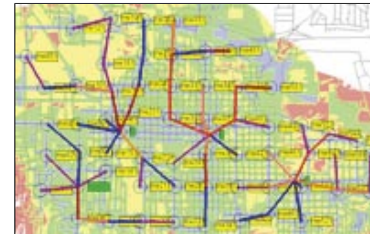
Mesh Routing display along with coverage from routers. Mesh link color selection determined by available data rate.
