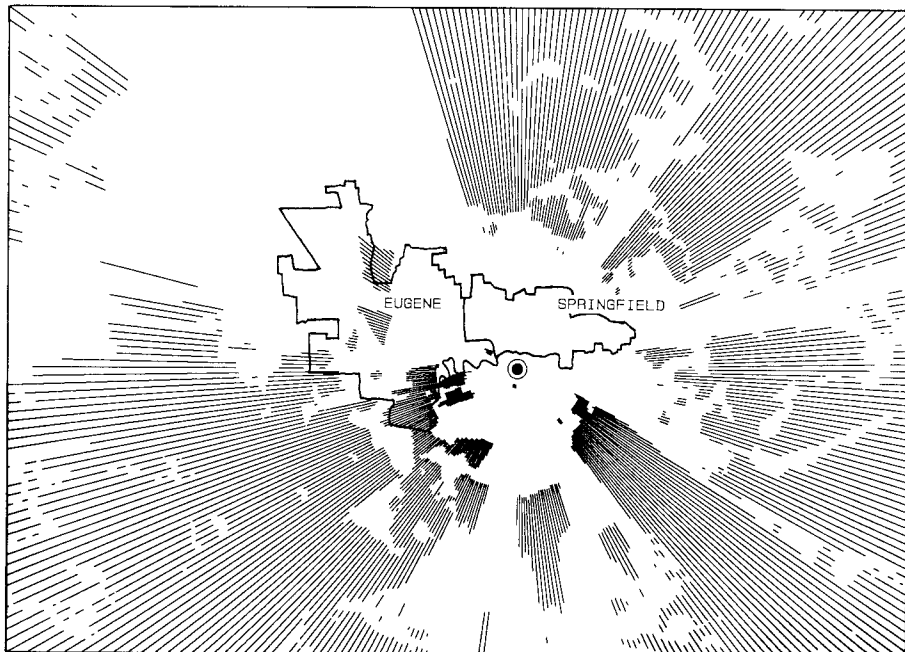
Figure 3c. Shadow map for the transmitter site on Quarry Hill. Shadow areas large over parts of Eugene.
